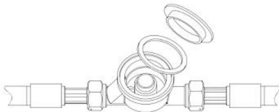
Mainfold blanking cap and O-ring of the meter man
