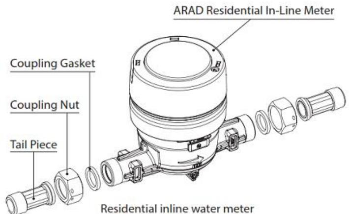
*DO NOT over tighten (TIGHTENING TORQUE SHALL NOT EXCEED 8 Nm for a 3/4" nut, and 17 Nm for a 1" nut). Do not use pipe dope or sealants.*
